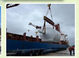
HLI coordinated, the collection and delivery of a TAD roll, which is a Through Air Dryer, Hoods and accessories for delivery to the Port of Portland, Maine (ME), for their onward journey to Tokyo. On the date determined by the customer, HLI's team arrived at the customers plant in Biddeford, ME. TAD Roll was lowered onto a 3 Bed Goldhofer transport trailer received the TAD roll. It was lowered onto the Goldhofer trailer by utilizing the customers on site overhead indoor crane.
