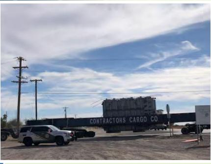
This job required the delivery of one 208,300 Lb. transformer from Laredo, TX to Coolidge, AZ. HLI was able to obtain all of the necessary permits and permissions to move the transformer from the transload facility, up to the final point of delivery inside the substation. Delivery was made easier by the use of an overhead crane, to lift the transformer from the railcar to the awaiting 19-axle girder transport trailer.
