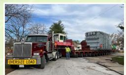
HLI railed this 500,590 Lb. unit from the manufacture in Mexico. all the way North to Van Meter, Iowa. After arriving at the rail siding of choice, HLI's crew inspected the unit, commenced removing all securing materials, began building the landing for the transformer and the bridge for the jack-and-slide system, to facilitate the unloading and transfer of the transformer from the railcar to the over the road transporter.
