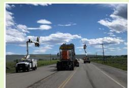
This 285,755 Lbs. transformer crossed the border from Mexico to the United States via HLI Laredo's transload facility, which is strategically situated near the Mexican border with the United States. HLI railed the unit 1760 miles to a rail siding located in Twin Falls, ID. HLI's rigging crew met the unit, and after the initial inspection, the GPS tracking device was removed, they then began releasing the transformer from the railcar.
