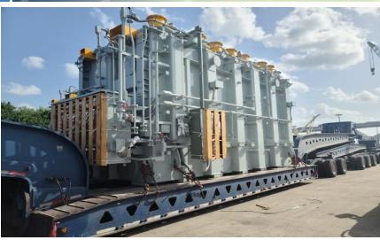
In August 2021, HLI coordinated the delivery and installation of four 261,600 Lb. transformers from the Port of Houston, to Throckmorton, TX. After HLI's crew arrived at the port, they began transloading the first transformer from its temporary staging area to an over-the-road transport trailer, for the final delivery to the customers substation. The most efficient, and economical method for transloading these heavy transformers from the staging area, was to utilize the jack-and-slide system.
