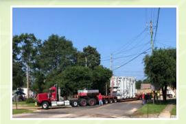
This 214,050 Lbs. transformer crossed the border from Mexico to the United States via HLI Laredo's transload facility, which is strategically situated near the Mexican border with the United States. HLI railed the unit 760 miles to a rail siding located in Hattiesburg, MS. HLI's rigging crew met the unit, and after the initial inspection began releasing from the railcar.
