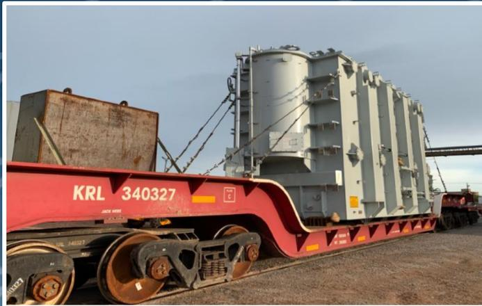
HLL employed a depressed center flat railcar to transport this 327,155 lb transformer from the transload border crossing in Laredo, TX to a rail siding in Clinton, OK. After inspecting the unit on arrival, work began to remove the securements from the transformer. At the rail spur, the rigging crew jacked-up the transformer and moved it across slides to a specialized 8-axle Goldhofer, HLL's crew then began the transportation to the final site.
