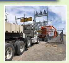
HLI railed this 227,400 lbs. unit 2,1357 miles from Tula, Mexico, to a rail siding in Blackfoot, Idaho, where it was met by HLI's rigging crew. Upon arrival, the transformer was inspected for damage, before cutting the securements that had held it on its long rail journey. The laying out of the jack-and-slide equipment commenced. The crew jacked the transformer up off the railcar, and transloaded the unit over to the dual lane trailer.
