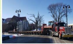
HLI railed this 300,8840 Lb. unit from the manufacture in Mexico, all the way North to Marshalltown Iowa, in the dead of winter. After arriving at the rail siding of choice, HLI's crew inspected the unit, commenced removing all securing materials, began building the landing for the transformer and the bridge for the jack-andslide system, to facilitate the unloading and transfer of the transformer from the railcar to the over the road transporter.
