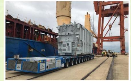
This 497,500 Lbs transformer was shipped from Altamira, Mexico to the Port of Virginia. HLI's crew arrived at the port to inspect the unit, before unloading commenced. After inspection, the unit was cleared and loaded to an awaiting Goldhofer trailer. Once secured, it began its journey to a temporary storage facility.
