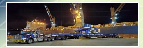
HLI transported a Yankee Dryer – a pressure vessel used in the production of tissue paper – 135 miles from the Port of San Diego, CA to Mexicali, MX. Dimensions of the unit were 19'07"L x 16' 09"W x 17'H, weighing 187,329Lbs. HLI chose a 19 axle trailer for the move. Once HLI's team had mobilized to the port, offloading of the Dryer commenced. The Dryer was transloaded from the ship to a specialized transporter.
