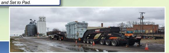
HLI railed this 257,000 lb unit from Laredo, TX to a rail siding in Lincoln, IL. After arriving at the rail siding, the transformer had to be offloaded from its heavy-duty railcar to an over the road transport system to be delivered to the substation. The best choice for offloading this heavy transformer from the railcar and loading the large transporter was using a jack and slide system.
