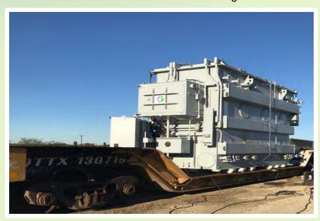
The transloading was repeated at the rail siding to offload the transformer from the road transporter. The cranes were assembled next to the railcar, then the transformer was pulled into position and safely loaded to the railcar. Welders then secured the transformer to the railcar. After inspection the railcar was cleared for moving.
