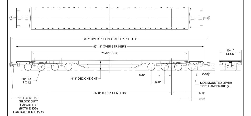
CAR WILL CARRY A CONCENTRATED LOAD AT THE CENTER OF THE CAR **EQUAL TO THE LOAD LIMIT**
