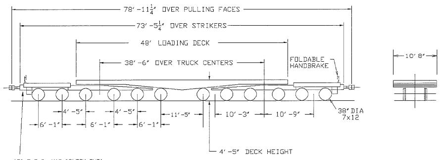
15" E.O.C. HAS "BLOCK-OUT' CAPABILITY (BOTH ENDS) FOR BOLSTER LOADS
