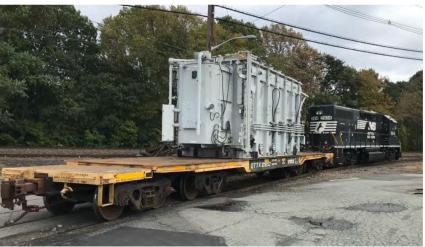
HLI railed this 265,000 lb. unit from Elizabeth, NJ to a rail siding in Bay, NJ. After arriving at the rail siding, the transformer had to be offloaded from its heavy-duty rail car to an over the road transport system to be delivered to the substation. At the rail spur, HLI employed an all-terrain crane to lift the transformer off the railcar and place it onto a specialized girder transport trailer for the subsequent haul to site.
