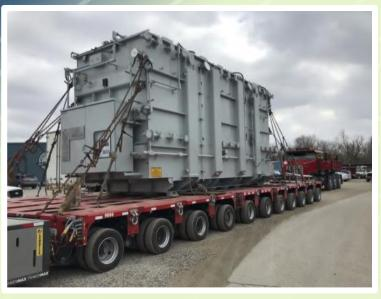
HLI was contracted a transformer from the Port of Entry, to a rail siding near the wind farm project located in El Reno, Oklahoma. After arriving at the rail siding, the transformer had to be offloaded from its heavy-duty rail car to an over the road transport system to be delivered to the substation.
