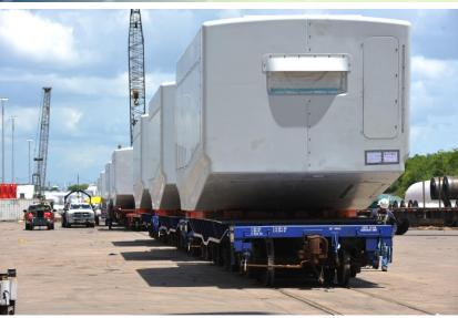
HLI was contracted to transport 95 Nacelles from the Port of Entry, to a rail siding near the wind farm project located in El Reno, Oklahoma. HLI worked with the local railroads to determine the best location to manage the transload. HLI identified two locations, one on the UPRR and one on the BNSF. Due to DOT highway restrictions, we utilized the TP&L facility in Enid, OK which is rail served.
