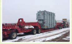
HLI railed two 190,000 lb units from Laredo, TX to a rail siding in Newcastle, UT. After arriving at the rail siding, the transformers had to be offloaded from their heavy-duty rail cars. to an over the road transport system to be delivered to the substation. At the rail spur, HLI employed an all-terrain crane to lift the transformer off the railcar and place it onto a specialized transport trailer for the subsequent haul to site.
