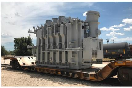
HLI was hired to ship this 156,746.Lb transformer from the factory in Mexico all the way up to Sandusky, OH.. The journey began deep in Mexico moving by rail. After arriving at the rail siding, the transformer had to be offloaded from its heavy duty rail car to an over the road transport system to be delivered to the substation. The best choice for offloading this heavy transformer from the rail car and loading the large transporter was using a jack and slide
