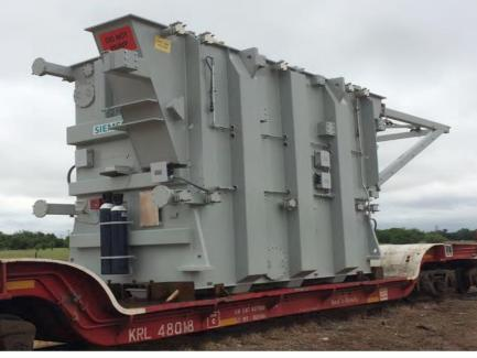
HLI railed this 198,049 lb unit 746 miles from Eagle Pass, TX, to a rail siding in Medford, OK. After arriving at the rail siding, the transformer had to be offloaded from its heavy duty rail car to an over the road transport system to be delivered to the substation. The best choice for offloading this heavy transformer from the rail car and loading the large transporter was using a jack and slide system.
