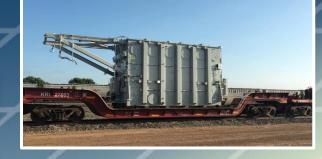
HLI railed this 206,592 lb unit from the US-Mexico border to its final destination in Beaver, OK. HLI received the unit secured on a railcar in Eagle Pass, TX. The unit then rode 611 miles of rail tracks to arrive at a rail siding in Beaver, OK. After the impact recorders had been reviewed, HLI's rigging crew removed the securements restraining the transformer and carefully jacked it off the bed of the railcar.
