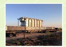
This 227,890 lbs transformer entered the United States on a railcar in Eagle Pass, TX. From there, HLI railed it 633 miles to a siding in Jal, NM. HLI's rigging crew met the unit at the siding, cut the lashings, and slid it off the railcar to a temporary structure of cribbing. The following day, the team loaded the transformer onto a specialized girder transport trailer for the over road haul to site.
