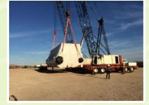
HLI engineered the trans-load of a 245,000 lbs. boiler from a girder trailer to a 6 deck 4 Goldhofer with prime mover at the Laredo, TX yard. The lift employed the services of HLI Laredo's 140 ton crane as well as their 200 ton crane. After the boiler had been safely set on a temporary foundation, the two cranes worked in cohesion to lift the girders from around the unit and set them to the side. The front and back trailers were then moved away to isolate the boiler on its temporary pad.
