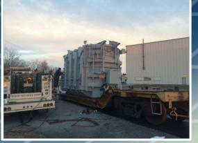
HLI received this 152,520 lbs transformer loaded and secured onto a 4 axle railcar in Laredo, TX. After the installation of GPS and impact recorder, the unit followed a northeastern route from its point of entry on the Mexico-Texas border to the town in New Jersey it was manufactured to call home. When the transformer had reached the rail siding in Flemington, NJ, the rigging crew lifted it from the railcar with a crane and loaded it onto a 3 deck 3 modular trailer.
